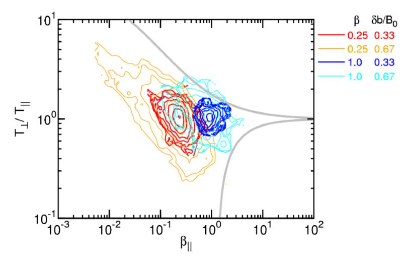
By varying parameters such as the level of fluctuations and the average plasma beta, Vlasov simulations "explore" distinct regions of anisotropy plane
